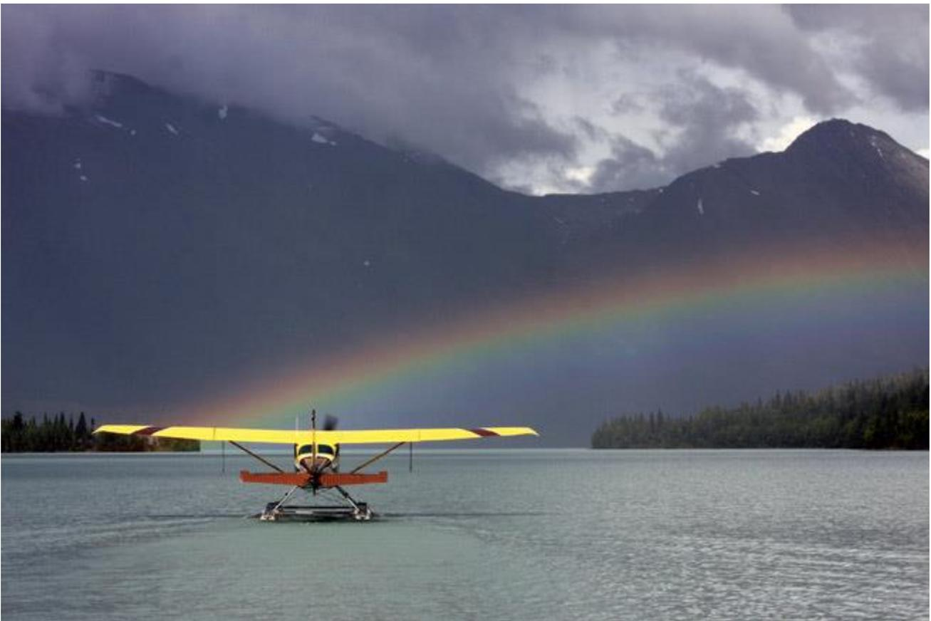
The stick is kept back to keep spray off the prop, as water can damage it almost like gravel. The Cubs are my first carbureted airplanes and I remember to turn off the carb heat; the water rudders need to come up before takeoff, and it's all going well until I add power and
